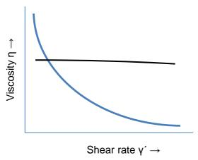
Typical "Newtonian" rheology: Viscosity remains constant regardless of shear rate. Compromise must be made when selecting balance of penetration and wash-off protection properties
